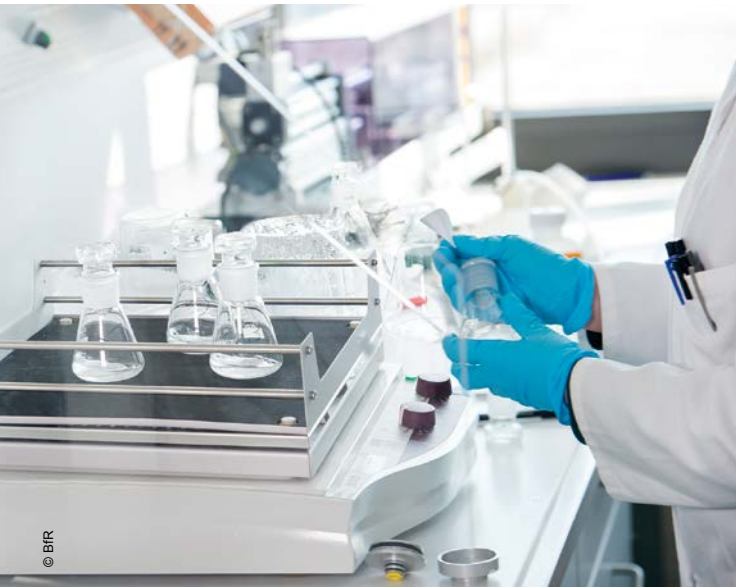
Shaken and checked: the vapour's components are extracted from the smoking machine's filter pad and then analysed.
