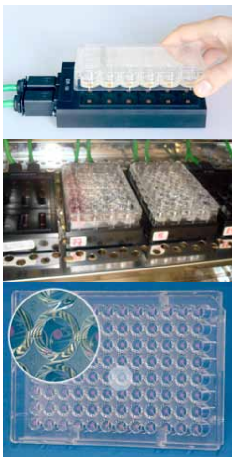
Figure 5. SensorDish reader with OxoDish (A). Setup of multiple OxoDishes connected in series in a humidified cell culture incubator (B). A 96-well Oxoplate (C).
