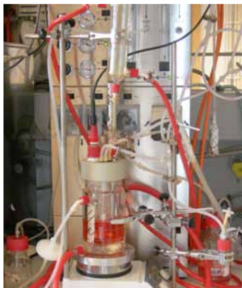
Figure 9. 3D bioreactor with fully controlled conditions.
