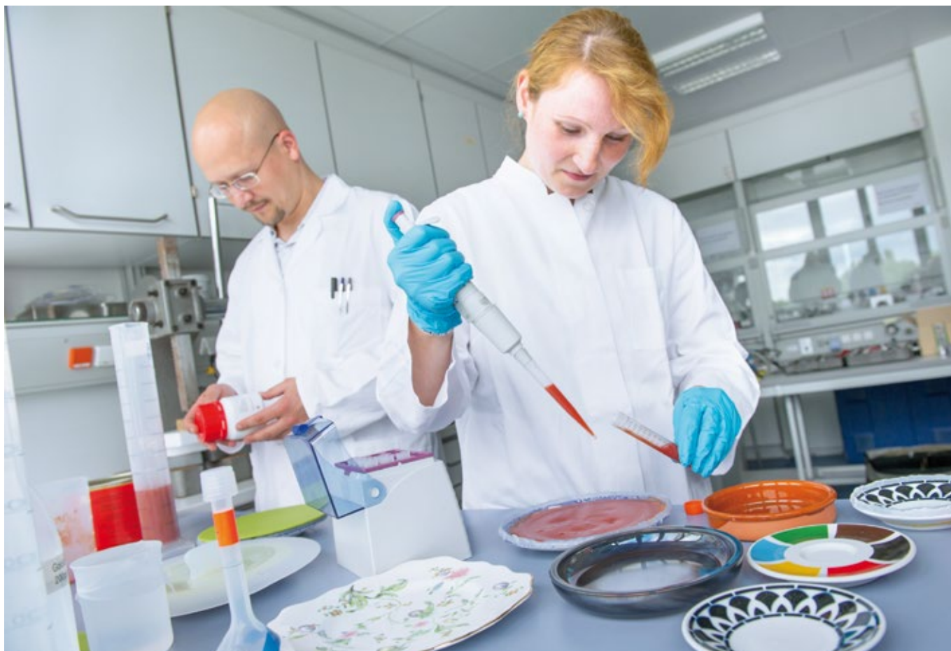
Staff at a National Reference Laboratory based at the BfR develop and validate analysis procedures to check the release of heavy metals from ceramics and glassware into food simulants.
